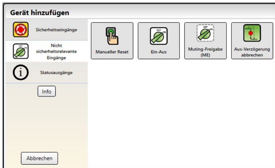
Figure 50: Non-safety-related inputs (virtual non-safety-related inputs only available via the Function view tab)
