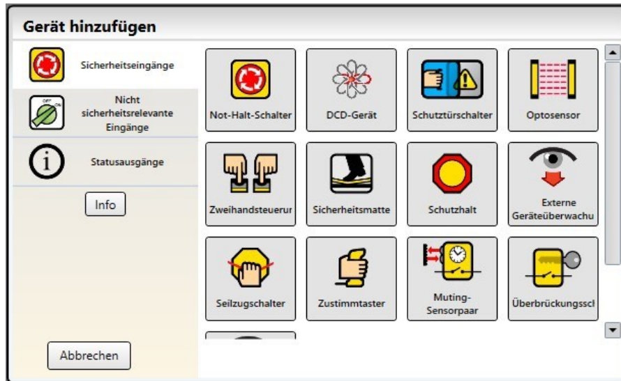
Figure 49: Safety inputs (virtual non-safety-related inputs only available via the Function view tab)
